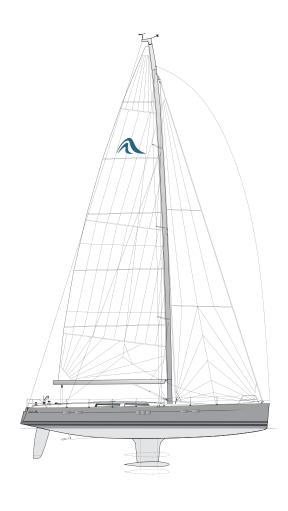
LOA 19.00 m | 62'4" Hull length 19.00 m | 62'4" LWL 17.10 m | 56′1″ Beam 5.20 m | 17′1″
